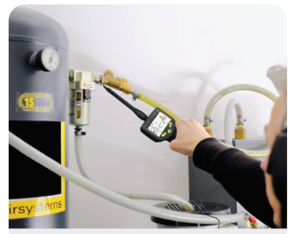
If needed, scan with the focus tube and focus tip till the exact location is found.
