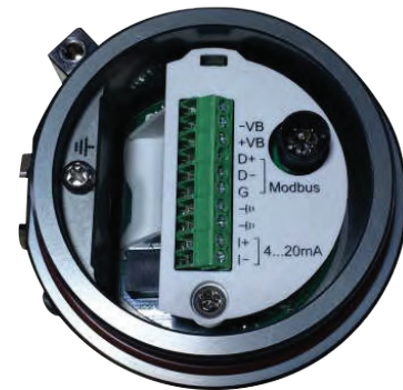
Screw terminals with signal labels inside the connection chamber
