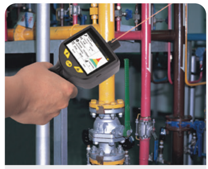
Point with the laser at an assumed leak. The display will show the level of the leak.
